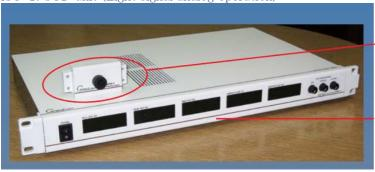
MPR-1A: PDAmodule to receive light signal
