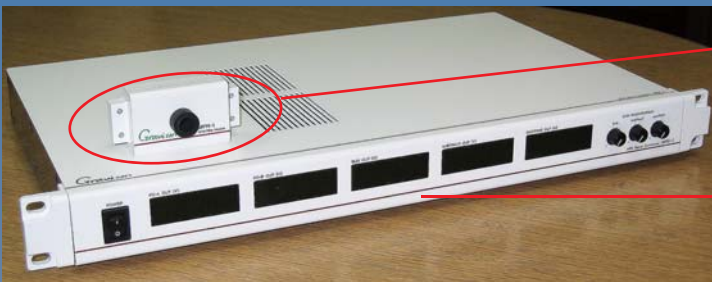
Top: MPR-1, PDA module to receive light signal
